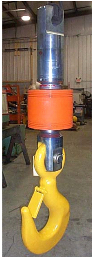
Insulated, 60T, NASA shuttle maintenance operations
